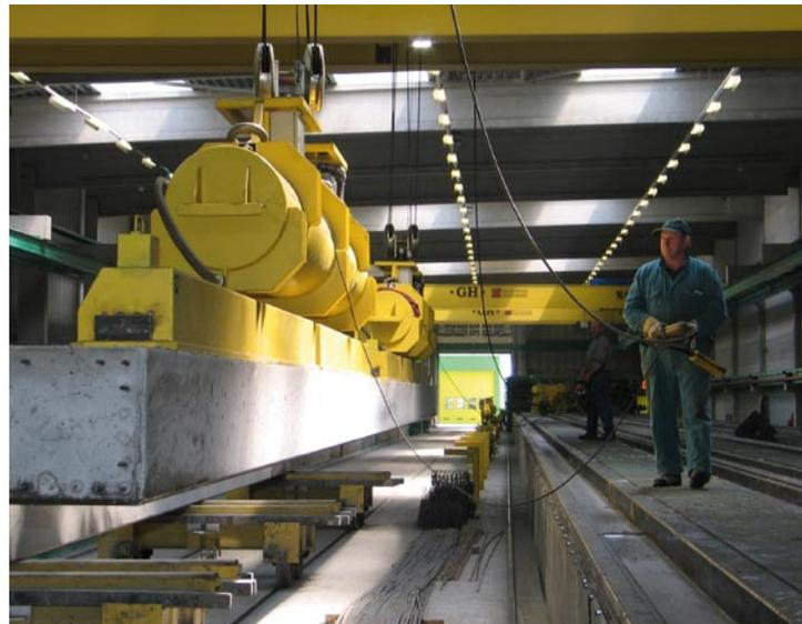
Precast concrete elements are factory made under strict controls. The manufacture of structural elements is automated to a considerable extent.
