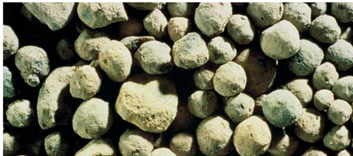
Image of a lightweight aggregate.
