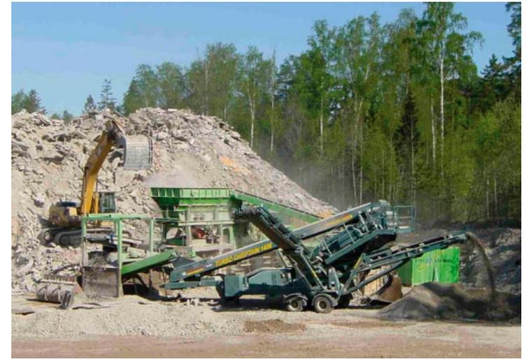
Concrete is as easy to crush and recycle as aggregate – almost 100% of a concrete building can be recycled, no matter how heavily reinforced.
